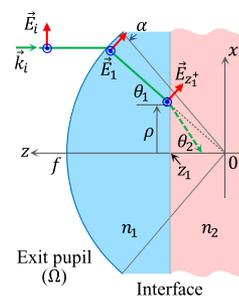
**Fig. 1.** Aplanatic focusing through a dielectric interface at  $z = z_1$ .  $f$ , focal length;  $\alpha$ , semi-aperture angle;  $(f, \theta, \phi)$ , spherical pupil coordinate;  $(\rho, \phi, z_1)$ , cylindrical interface coordinate.
