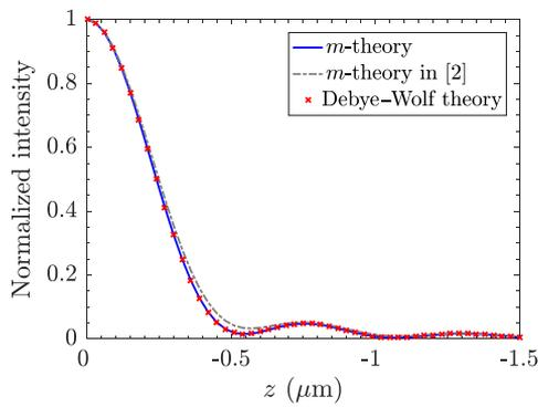
**Fig. 2.** Light focusing into an index-matched medium (oil  $n_1 = n_2 = 1.522$ ) at  $z_1 = 50 \mu\text{m}$ . The  $m$ -theory with correct apodization yields the same axial distribution by the Debye–Wolf theory.  $f = 1.8 \text{ mm}$ ,  $\text{NA} = 1.4$ , vacuum  $\lambda_0 = 488 \text{ nm}$ .
