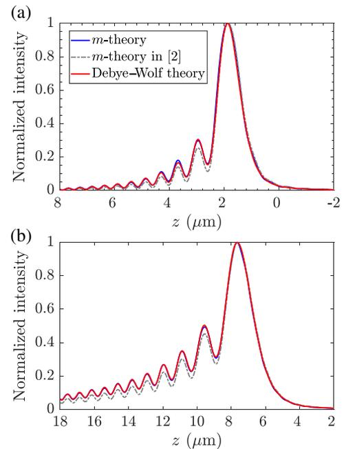
**Fig. 3.** Comparison of normalized axial intensity distributions if focused through a glass/water interface (1.522/1.337) at 1.4 NA.  $\lambda_0 = 488 \text{ nm}$ ,  $f = 1.8 \text{ mm}$ . (a)  $z_1 = 10 \mu\text{m}$  and (b)  $z_1 = 50 \mu\text{m}$ .
