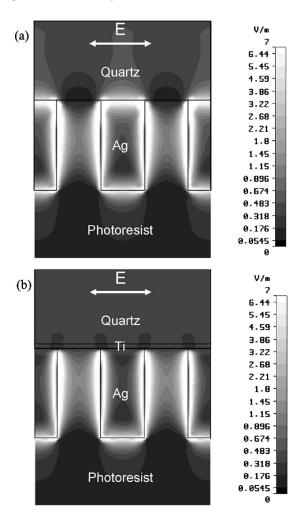
FIG. 2. (a) Simulated amplitude of *E*-field at the cross section of silver hole array; silver film thickness 40 nm, hole diameter 20 nm, periodicity 40 nm. (b) Silver hole array with titanium adhesion layer (3 nm) at the same condition as (a).
