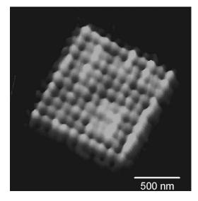
FIG. 4. AFM image of an exposure pattern on 120 nm period, where the hole size of 60 nm, the silver film thickness of 40 nm, the spacer layer thickness of 15 nm, and the exposure dose of 80 mJ/cm<sup>2</sup>.
