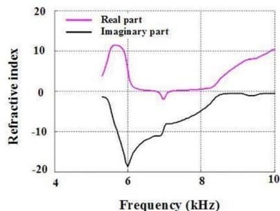
FIG. 5. (Color online) Effective refractive index of acoustic metamaterial consisting of hollow soft silicon rubber cylinders in water. The configuration is the same as presented in earlier figures. A narrow frequency band of negative index is seen around 7000 Hz. The negative index obtained is loss based, which is different from the double negative acoustic medium.
