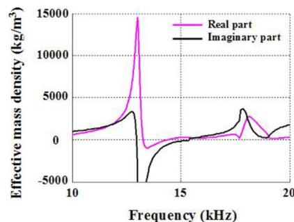
FIG. 6. (Color online) Effective mass density of an acoustic metamaterial consisting of rectangular rods of soft resin (2 mm height and 1.5 mm width) attached to rigid rods of the same dimensions in water. The unit cells are arranged in a square lattice with a lattice constant of 4 mm. A narrow frequency band around 13 kHz shows a negative effective mass density equal in magnitude to the density of water.
