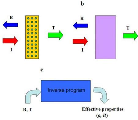
FIG. 1. (Color online) Technique used for obtaining the effective properties of a metamaterial. (a) This illustrates the system under consideration with incident, reflected, and transmitted plane waves. (b) This shows a slab of effective material equivalent to the system shown in (a) at a selected frequency. (c) This illustrates a technique used for obtaining effective properties of a metamaterial.
