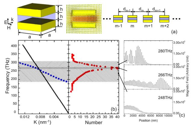
FIG. 1. (Color online) The geometry of a metallic trilayer structure, the magnetic field distribution at the magnetic resonant frequency, and the model of the graded nanosandwich chain are shown in (a). The effective dispersion relation and the propagation length of the chain are shown in (b), and the magnetic field localizations at three different frequencies are presented in (c).
