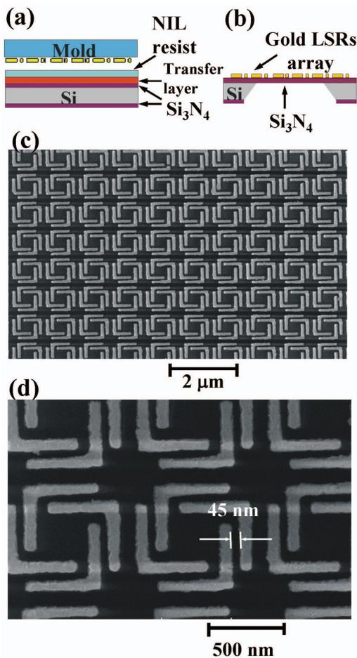
FIG. 2. (Color) (a) Illustration of the nanoimprint lithography procedure. (b) The schematic of LSRs on a  $\text{Si}_3\text{N}_4$  membrane. (c) SEM image of a fragment of the final LSR metamaterial (total size is about  $1\text{ mm} \times 100\text{ }\mu\text{m}$ ). (d) SEM image of LSRs demonstrating the smallest feature size of about 45 nm.
