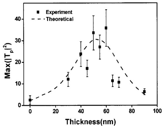
FIG. 4. Measured peak field enhancement  $|T_p|^2$  vs the thickness of silver films at  $\lambda = 514.5$  nm. The dashed line is the calculated value by Fresnel equation using  $\epsilon_{Ag} = -10.8 + 0.42i$ .
