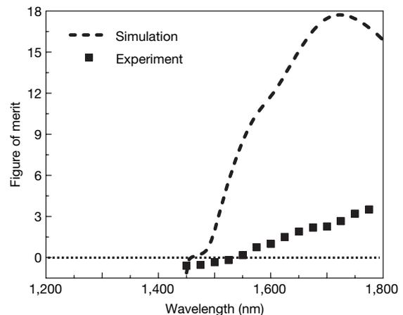
**Figure 5 | Figure of merit for the 3D fishnet structure.** Plot of FOM against wavelength for the simulation (dashed line) and experiment (squares). The lower experimental FOM is due to reduced transmission resulting from fabrication imperfections. The experimental FOM reaches 3.5 at 1,775 nm, where  $\text{Re}(n) = -1.23$ .
