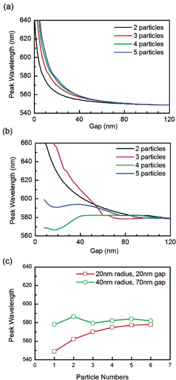
**Figure 3.** (a, b) Peak wavelengths of the scattering spectra calculated by using the T-matrix method for finite 1D chain of Au nanospheres with 40 nm diameter (a) and 80 nm diameter (b). (c) Peak wavelengths vs chain lengths for 40 nm particles with 20 nm gaps and for 80 nm particles with 70 nm gaps.
