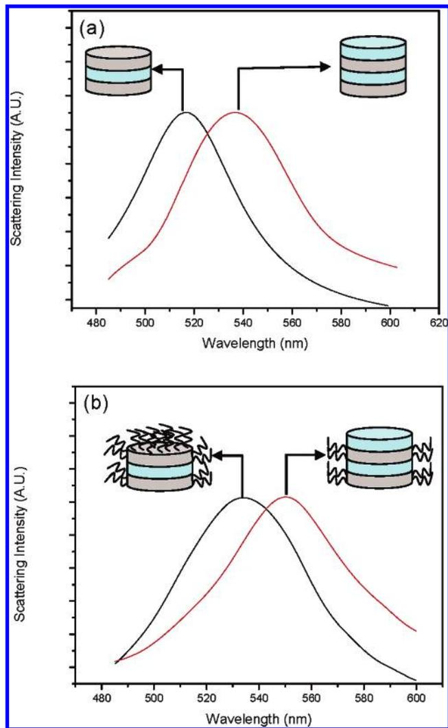
**Figure 2.** (a) Measured scattering spectra for an individual TNPR and a capped TNPR before *pMA* incubation. The Ag and SiO<sub>2</sub> layer thicknesses are 20 and 5 nm, respectively. (b) Measured scattering spectra for an individual TNPR and a capped TNPR after 100 μM *pMA* incubation for 24 h. The curves were normalized such that the maximum peak positions are identical.
