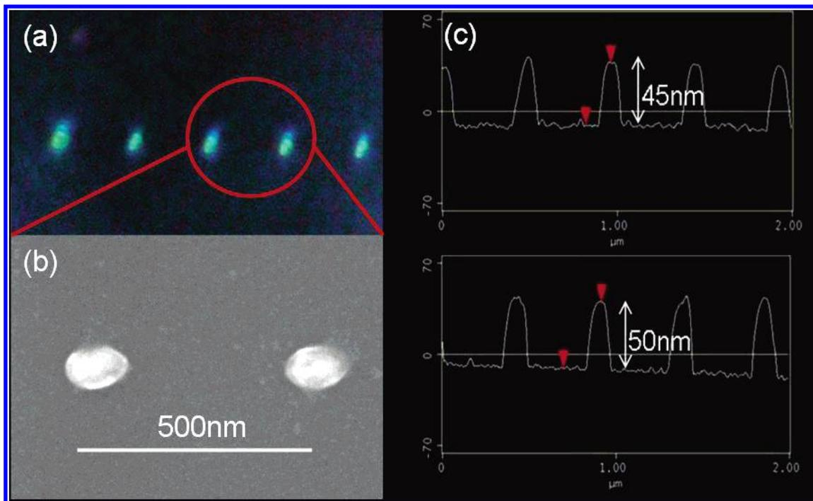
**Figure 1.** (a) Real color picture of TNPRs illuminated by evanescent white light waves taken with a digital camera. (b) SEM image of a Au/SiO<sub>2</sub>/Au three-layered TNPR singlet. (c) AFM measurement of a TNPR and a 5 nm SiO<sub>2</sub>-capped TNPR. The measured height difference shows that a 5 nm SiO<sub>2</sub> layer was successfully deposited on top of the metal surface while a shadow mask was inserted over the TNPR to prevent SiO<sub>2</sub> layer deposition.
