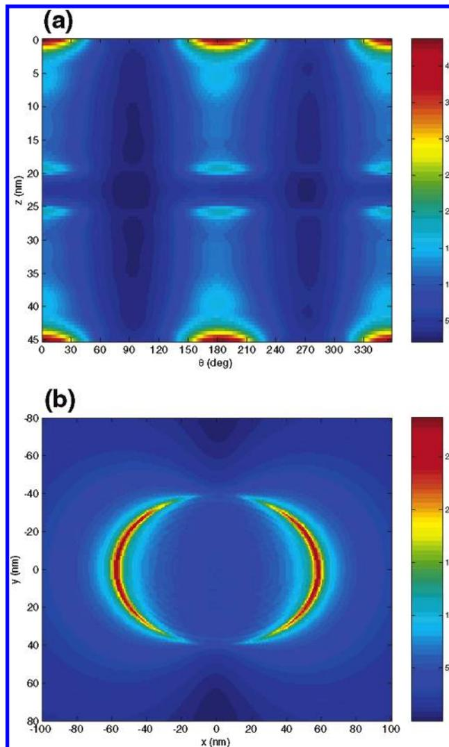
**Figure 4.** (a) Amplitude distribution of the total field computed just outside the side of the curved cylindrical surface. (b) Amplitude distribution of the total field computed above the top TNPR metal surface.
